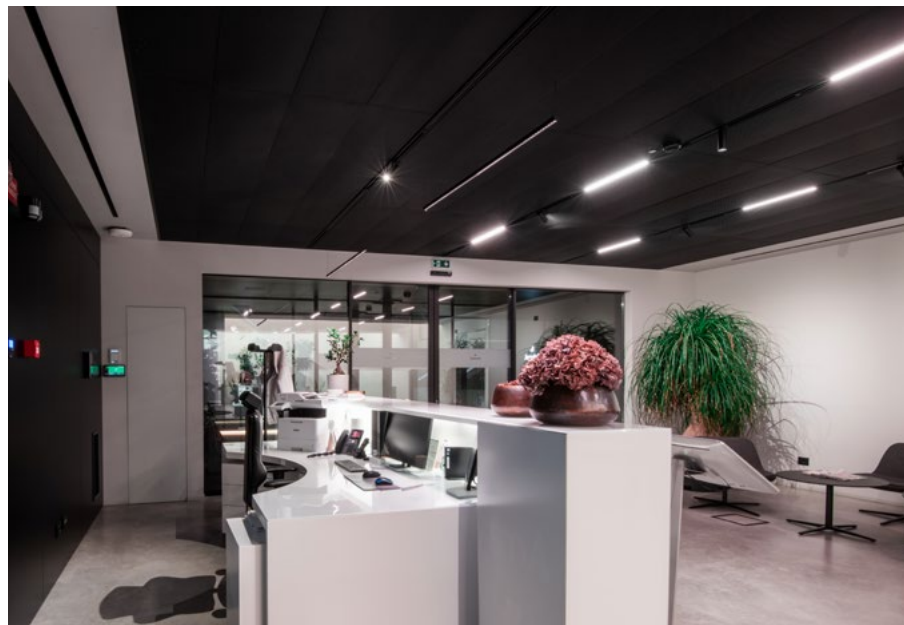
Vert Occulto 600x1200 mm in galvanised steel with post-painted finish, with Ø2mm perforation and non-woven fabric fleece for increased acoustic comfort.
